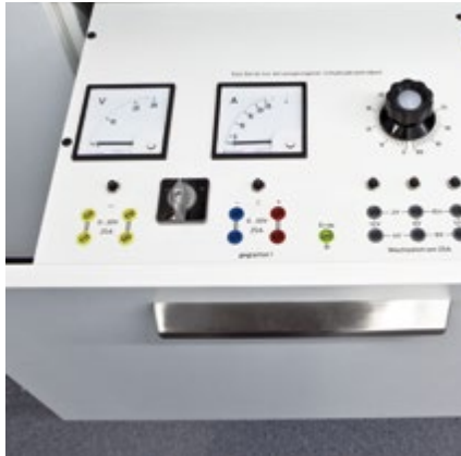
The optionally integrated electrical power supply unit passes on the voltage selected by the teacher to the pupils.
